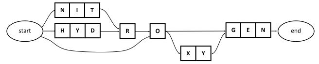
This DAWG correctly recognizes the letter sequences NITROGEN, HYDROGEN, and OXYGEN, but it also incorrectly recognizes the letter sequences NITROXYGEN and HYDROXYGEN, which were not intended.
